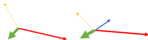
Fig 2 Illustration for finding corresponding vectors (each color is corresponding result). Searching from the pair of vectors with maximum product, remove the pair then search maximum product again until one bifurcation has no more vectors
